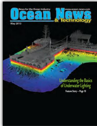
Harakka island pier in front of Helsinki. Underwater data collected with Reson and above water captured by Riegl laser scanner installed in Meritaito's unique mobile survey platform.
