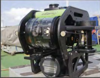
LBV300-5 - versatile dual vertical thruster ROV system.
